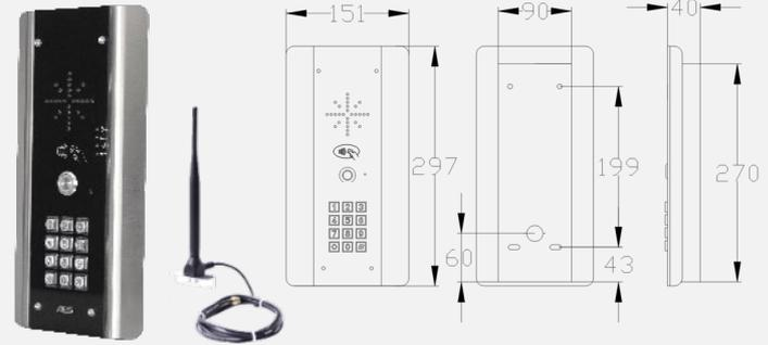
Stylish, modern curved profile call point with blue backlighting effect and illuminated keypad option. Constructed from 100% marine grade stainless steel and toughened black gloss acrylic faceplate with integrated Prox reader. Kits complete with 3 proximity cards/tags. Non-Keypad & Keypad Models.
