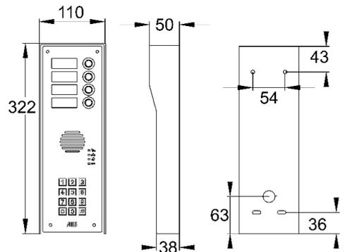
Panels are available in all black with textured powder coated aluminium hood and gloss acrylic faceplate or full BS316 marine grade stainless steel. Both panels has white illuminated push button and keypad. Up to 4 call buttons (each button calling a different home owner).
